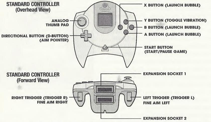
Never touch the Analog Thumb Pad or Triggers L/R while turning the Sega Dreamcast power ON. Doing so may disrupt the controller initialization procedure and result in malfunction.
